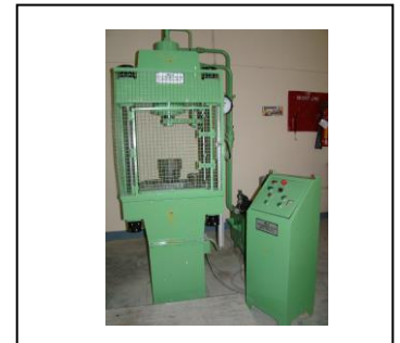
Digital photograph of uniaxial press used for pulleys compaction
